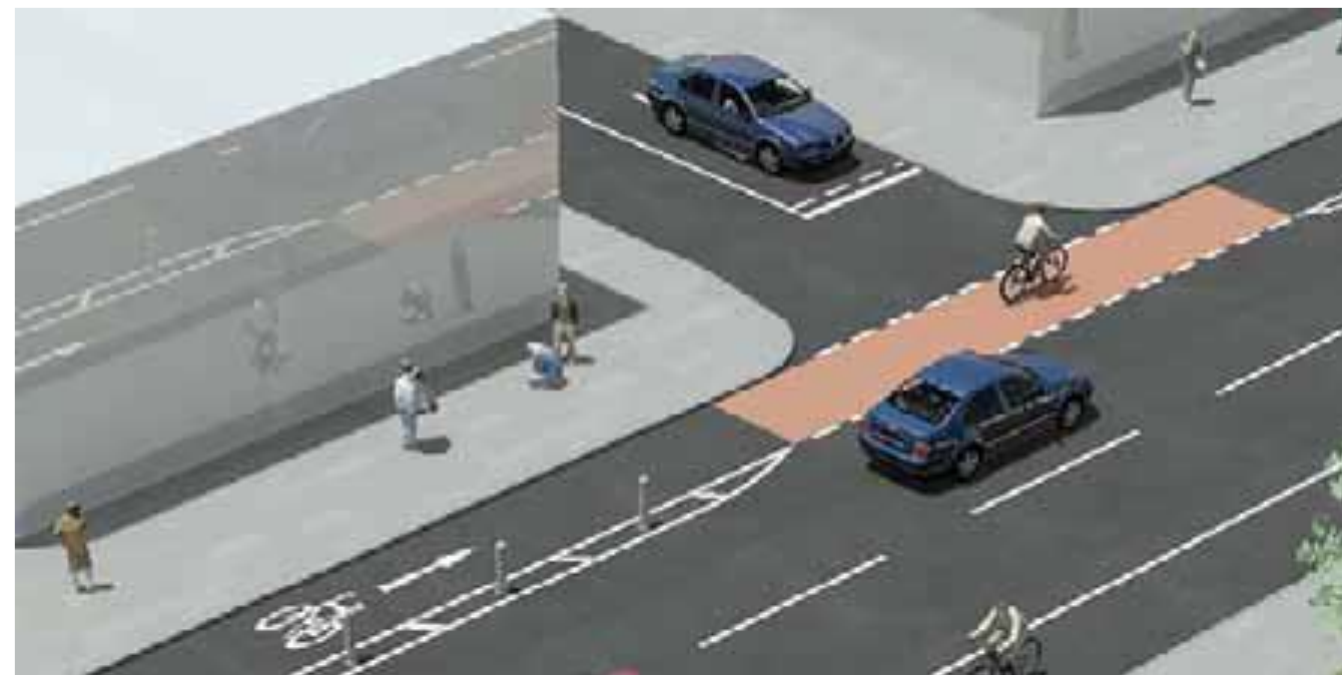
Figure 32: On-Road Cycle Lane Priority Junction Treatment
